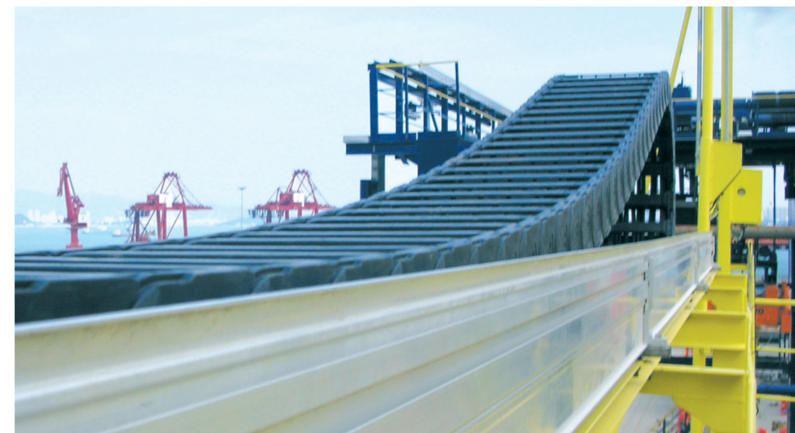
Seawater-resistant aluminium SuperTrough for an igus® E4 system on an RTG crane
